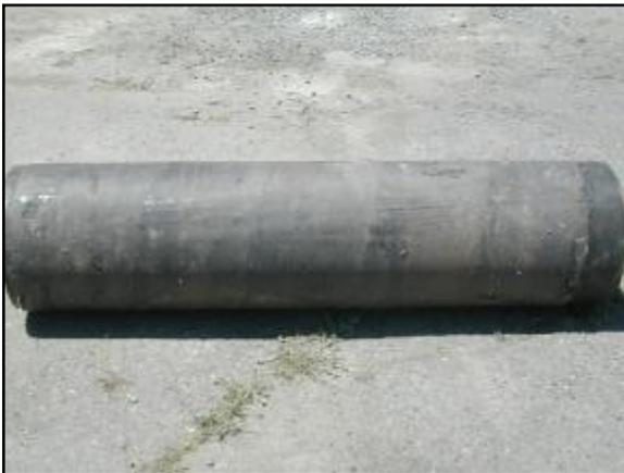
**Detail of Tape Wrapped Steel Pipe After 35 Years of Service. No Signs of Deterioration.**
