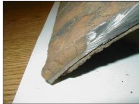
**Detail of Graphitized Ductile Iron Pipe at Perforation of Sewer Force Main**
