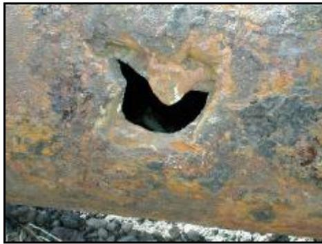
**Detail of Perforation of Ductile Iron Sewer Force Main After Approximately 20 years of service**
