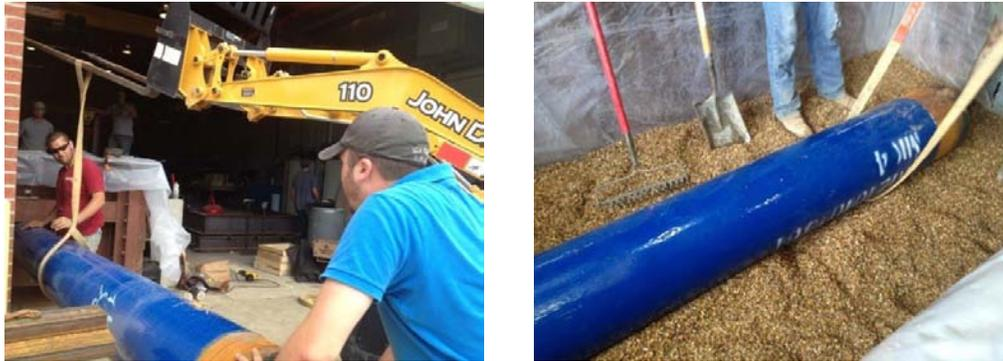
**Figure 4: Placing of the Polyurethane Coated Pipe inside the Soil Box**
