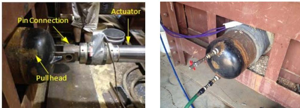
Figure 11: Fabricated Pull-head welded to host pipe (left); water supply line attachment to rear cap (right)
