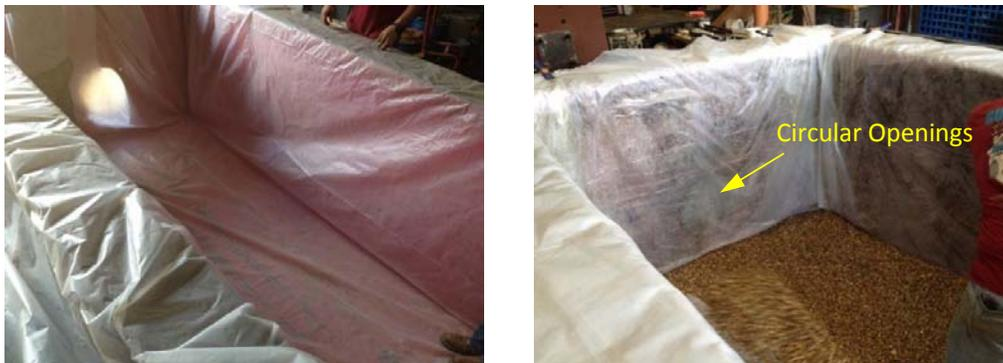
**Figure 3: Soil box covered by Polyethylene sheet on all sides (left) and soil box filled with pea gravel (right)**
