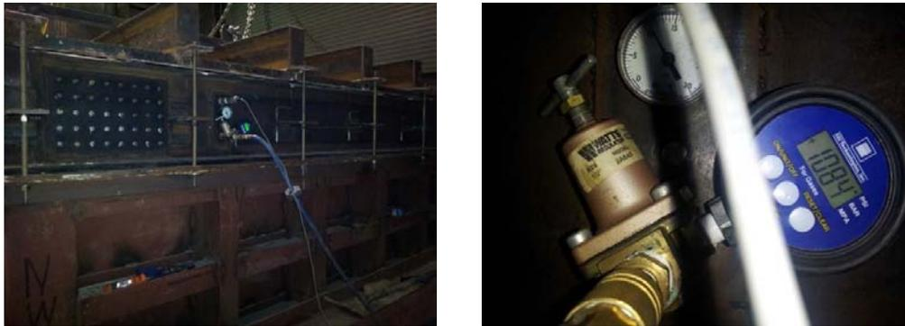
Figure 10: Pressure applied to the soil box (left); Pressure reading on the gauge (right)
