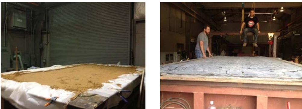
**Figure 6: Soil chamber filled with Sand(left); Rubber bladder on top of the soil's surface (right)**
