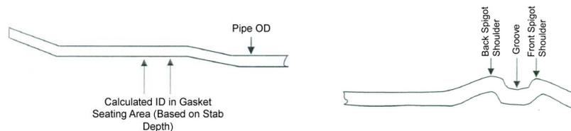
**Figure 6a, b: Critical Bell Dimensions, Spigot Dimensions**
