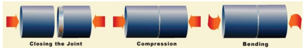
A 60-inch outside diameter Permalok Casing Pipe, with a wall thickness of 0.625-inch, will require approximately 40 to 60 tons of compressive force to complete the connection.
