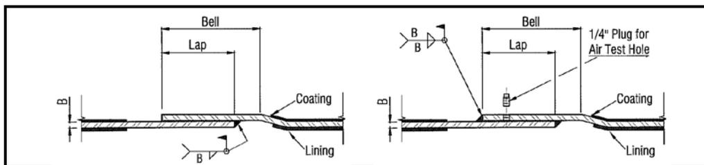
Figure 3a, b: WSP w/ Single, and w/Double Lap Welded Slip Joints
