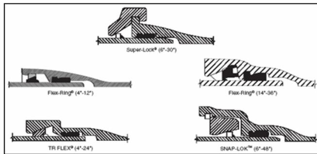
Figure 1: Proprietary Restrained Joints for DIP
