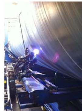
Figure 2a, b: Spiral-Welded Steel Pipe (AWWA 2004), Plasma Torch for Cutting Cylinders to Appropriate Lengths
