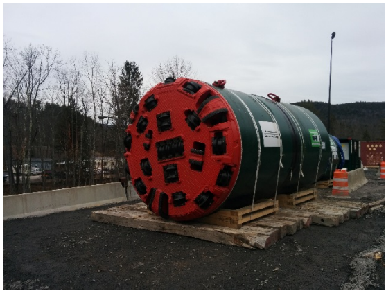
Figure 6a. Microtunnel Boring Machine
