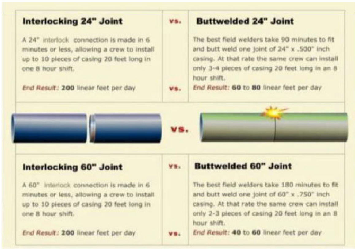
Figure 5. Interlocking Joint vs Welded Joint
