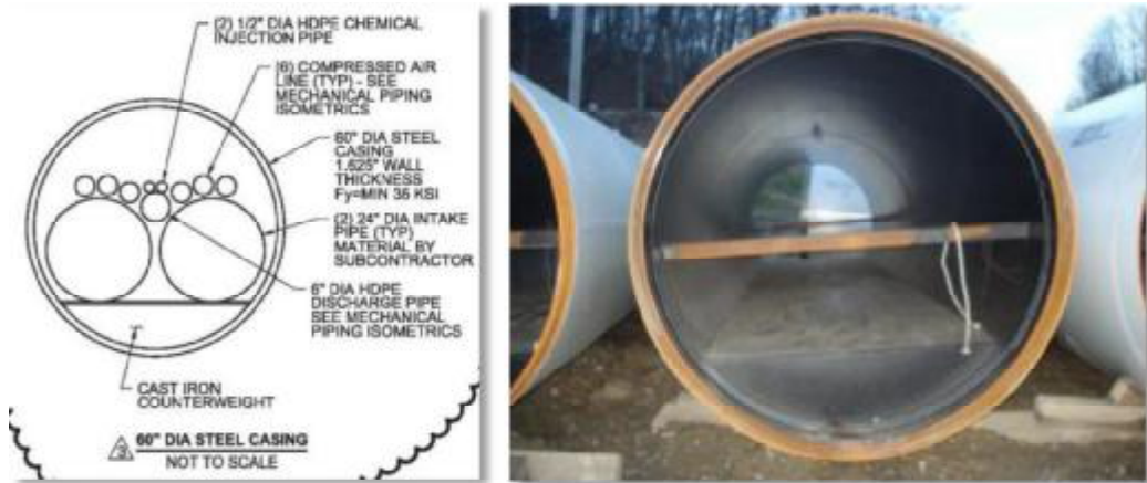
Figure 7. Cast Iron Ingots for Buoyancy
