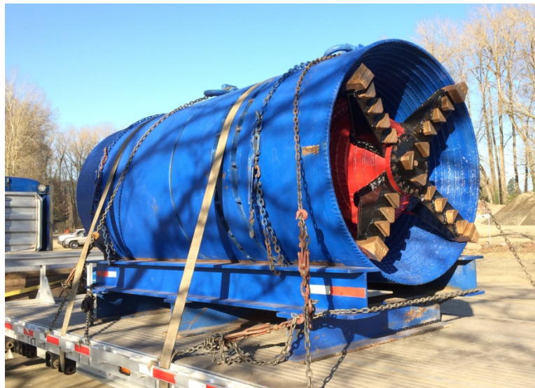
Figure 5: Iseki TCC 1200 Unclemole® MTBM Used for Microtunneling Across OR-99E
