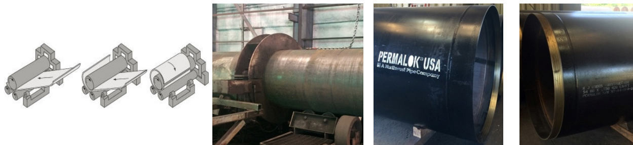
7a, b, c, d: Cylinder Rolling, Jig for Alignment During Girth Seaming Welding, Completed Permalok® Casing
